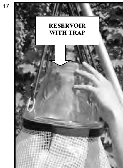
Slide the trap with the reservoir attached into the ring and fasten the suspension rubber to the ring again with the harp shackle. Now attach the wind rubber for extra strength and wind resistance.
